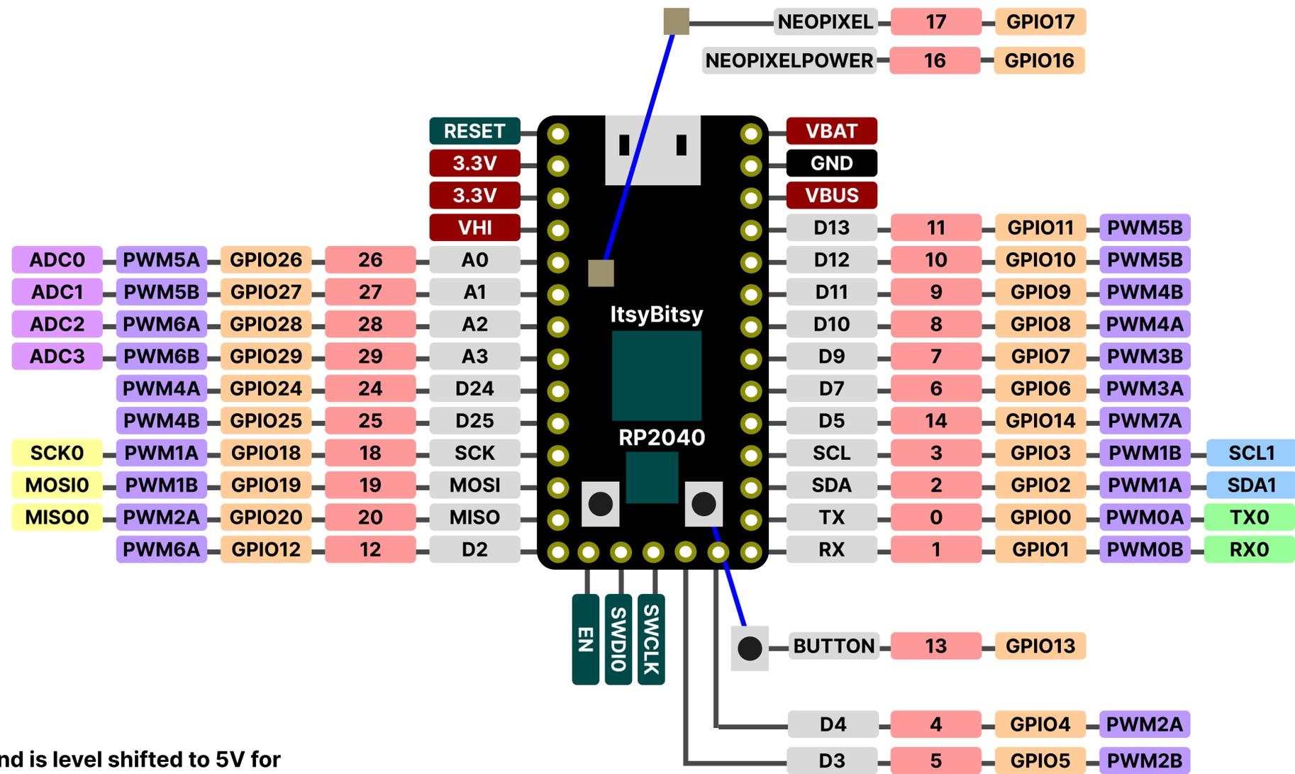
Pin D5 is an output only and is level shifted to 5V for driving Neopixels, etc.
